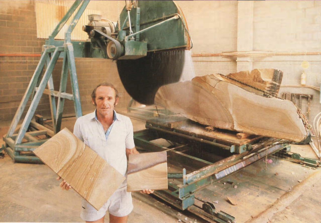
Sandstone blocks being cut to make tiles, Helidon Sandstone factory, Bethania
