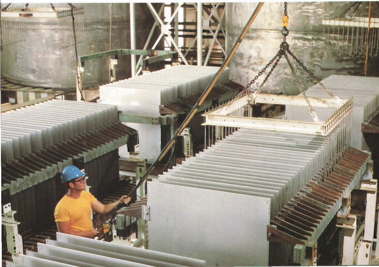
Preparing stainless steel starter sheets, Townsville Copper Refinery
