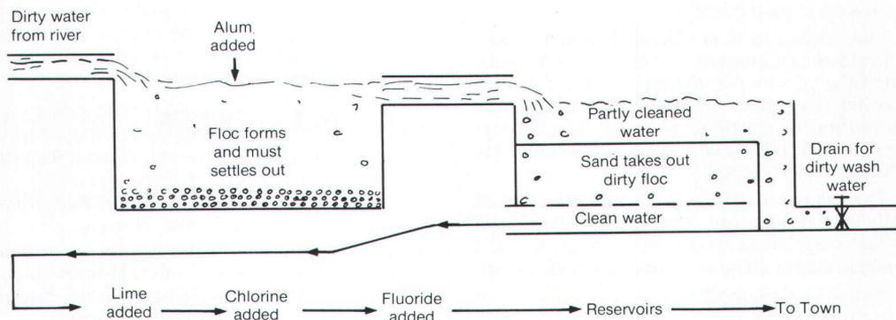
When coagulation is complete, dirty floc is suspended in clean water. By flowing the water slowly through settling basins most of the floc settles out and is run off to waste. The settled water is run through filters to remove the last traces of floc.
