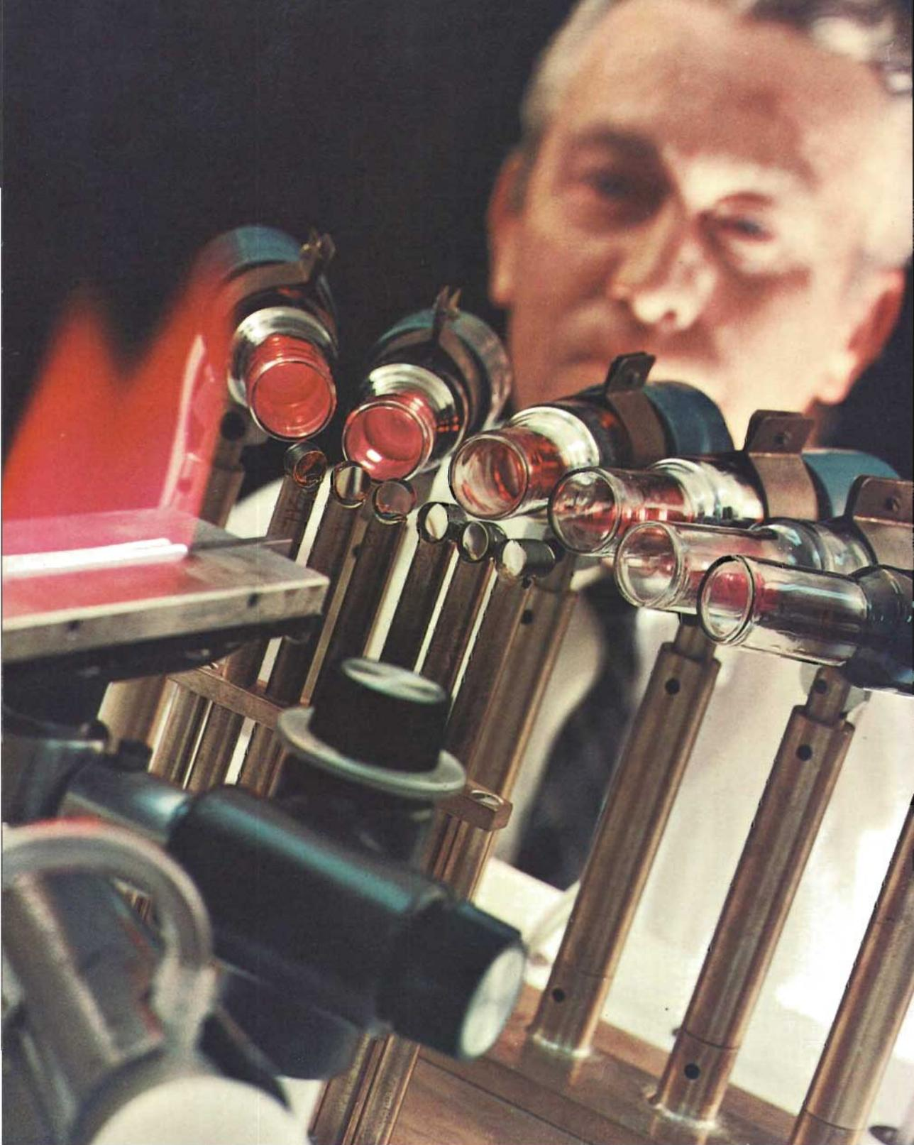
The atomic absorption spectrometer developed in Victoria by the C.S.I.R.O.
