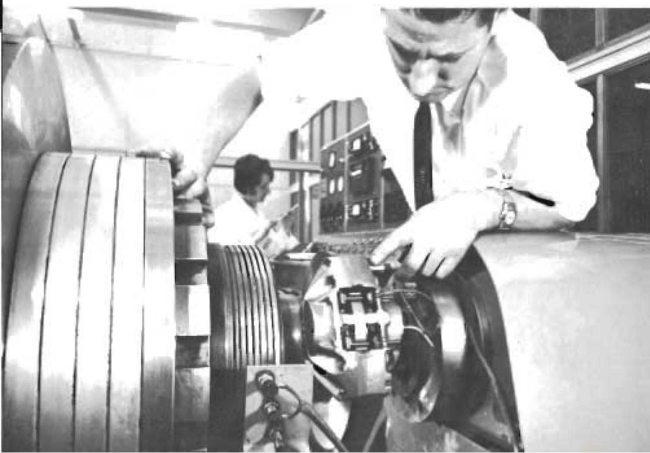
Setting up a disc brake assembly on a heavy duty inertia brake dynamometer for a high speed test.
