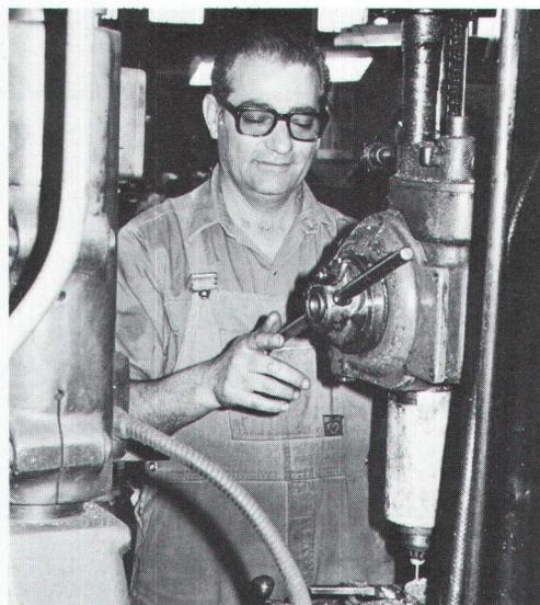
*Drilling a sub-assembly for bit brace manufacture*
