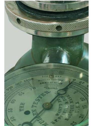
A Mullen Burst Testing machine, patent 1909, used to measure how much pressure could be applied to fabric before it burst. This is still used as a measure of fabric quality.
