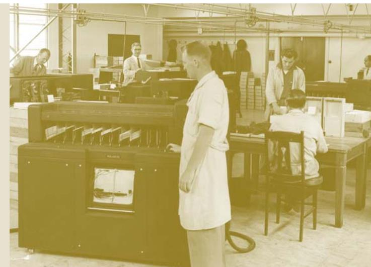
Mechanical tabulation equipment used for the 1954 census. A sorting machine is in the foreground.
