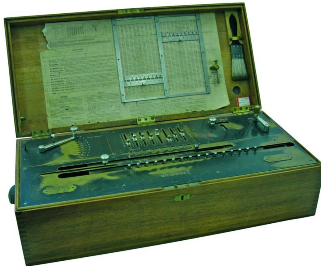
at an experimental stage and would have required considerable modifications to be suitable for Australia. However, Burroughs' Adding Machines were used for tabulations by locality and a Millionaire calculating machine was also used. Unlike other adding machines of the period, the Millionaire could do multiplication. The Millionaire involved relatively new technology and this machine was one of only a couple of thousand in the world at that time.
